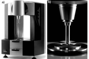
Fig. 2. Rotational rheometer Kinexus Pro: a) main view, b) testing node
