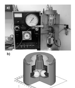
Fig.1. Four-ball testing machine by Roxana: a) main view, b) friction node
