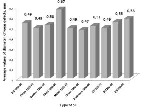
Fig. 3. Specification of wear defects of engine oils tested by ASTM D2266-01
